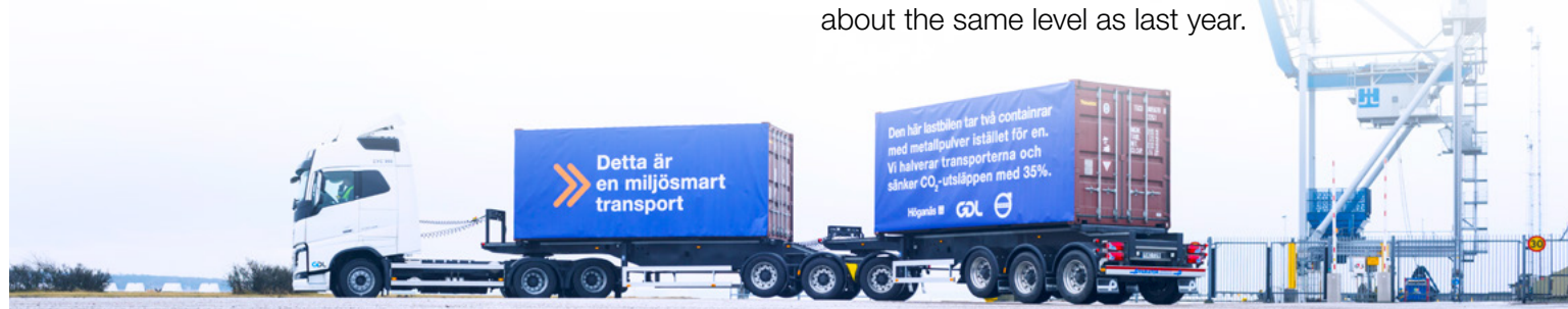
HCT transport vehicles can carry two freight containers instead of one, which lower carbon dioxide from our transports.
